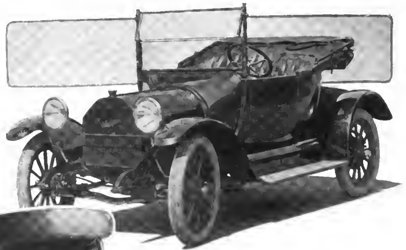
Above—Three-quarter of Studebaker four-cylinder, three-passenger roadster for 1915. Two of the passengers sit at the driver's right, the driver's seat being slightly in advance of the seat for the other two. Note the broad doors and ample storage space in the rear
